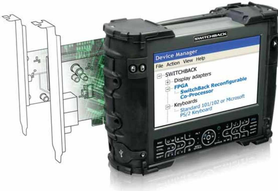
Figure 3 – Any reconfigurable hardware expressed in the FPGA can connect to the main processor, which can access it as though it were physical hardware plugged into an expansion port.
